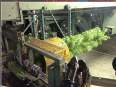
In the next step, different machinery takes in the long run of foliage and begins to cut and build it into thick garland lengths.
