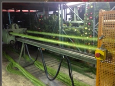
Our in-house machinery cuts and winds rolls of PVC vinyl into lengths of foliage to fashion into garlands, wreaths, sprays, trees and branches.
