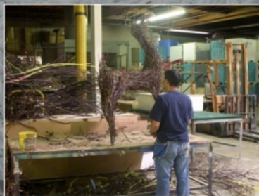
Next, they apply the cut Manzanita twigs artistically by hand to the framework, ensuring to fill in the piece completely.
